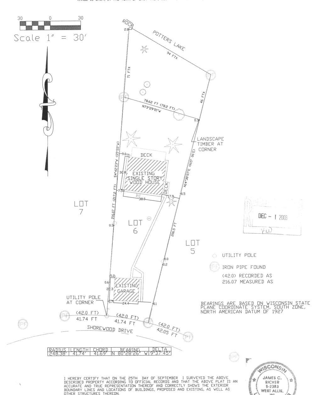
I HEREBY CERTIFY THAT ON THE 25TH DAY OF SEPTEMBER I SURVEYED THE ABOVE DESCRIBED PROPERTY ACCORDING TO OFFICIAL RECORDS AND THAT THE ABOVE PLAT IS AN ACCURATE AND TRUE REPRESENTATION THEREOF AND CORRECTLY SHOWS THE EXTERIOR BOUNDARY LINES AND THEOREMS. THEREBY AND THE PROPERTY OF BUILDINGS, PROPOSED AND EXISTING, AS WELL AS OTHER STRUCTURES THEREON.
